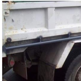
Rope rails give many options for tie-down.
