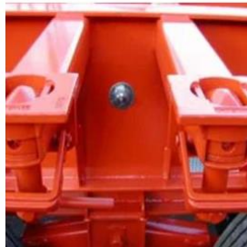
For restraint of containers generally twist locks (various types) or twist lock pockets are used.
