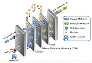
Schematic diagram of a fuel cell and the chemical reactions that take place inside it. Image retrieved from <a href="https://i.pinimg.com/originals/0d/62/9c/0d629cd17632ae1da57b3436327d556f.jpg">https://i.pinimg.com/originals/0d/62/9c/0d629cd17632ae1da57b3436327d556f.jpg</a>
