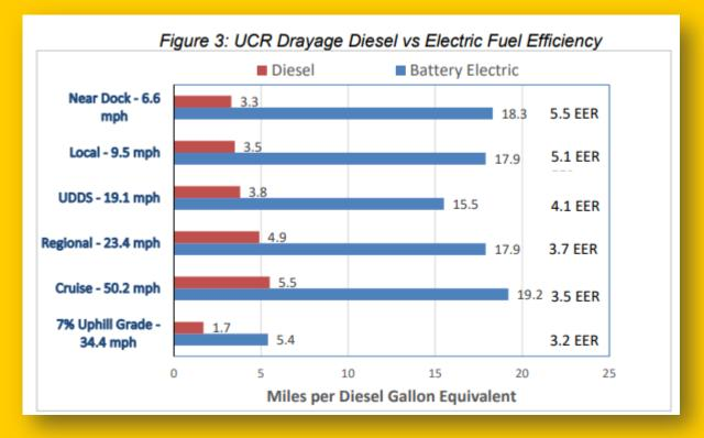
Battery Electric Truck and Bus Energy Efficiency Compared to Conventional Diesel Vehicles California air Resources Board 2018
