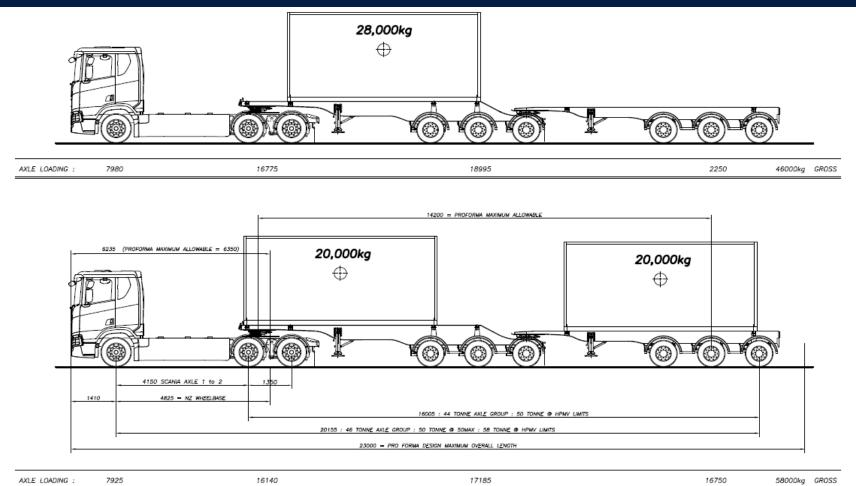
\*\* NOTE : COMBINATION GROSS OF 58 TONNE ASSUMES 50T AXLE 3 TO 9 LIMIT PLUS 8.0 TONNE\* LIMIT ON STEER AXLE / 17 TONNE\* LIMIT ON DRIVE AXLES \* SUBJECT TO APPROVAL FOR EV TRACTOR
