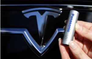
Over 7,000 Panasonic 18650 cells are integrated into the Tesla Model S battery pack
