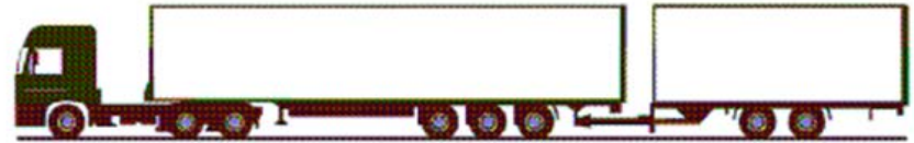
Tractor + semi-trailer + center axle trailer
