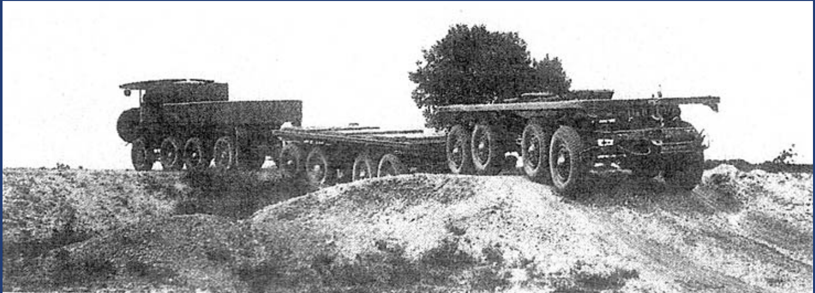
The AEC Government Road Train is shown here being checked on a rough track at the British Army proving grounds before being shipped to Australia in 1934. It was loaded with heavy steel plates for the trial. ( The Engineer )
