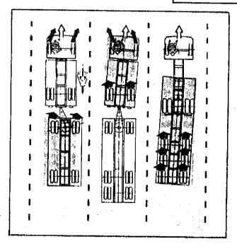
Rear axie should always sit at 90 degree angle to frame. Deviations male truck want to go off road and can also create illegal situation because truck takes up more space than maximum legal width.
