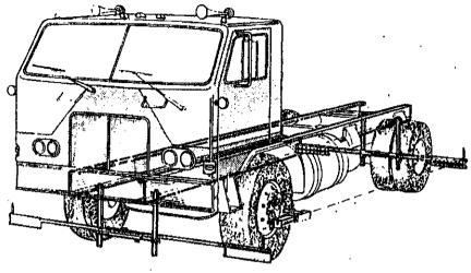
Left: Scales are located at both ends of truck so that entire vehicle length is used as measuring reference, resulting in extremely accurate readings.
