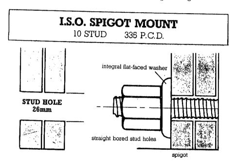
As more clamping force was needed to resist higher engine and braking torque the spigot mount or hub piloted disc wheel was introduced. All of the later model European and Japanese heavy commercial vehicles reaching our market are fitted with this wheel which complies with International Standard 150-4107.
