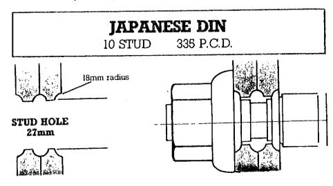
Disc wheel summary - when replacement wheels of any type are supplied by a dealer to a fleet, a check should be made to compare the stud hole drilling of the wheel with that of the old one, to ensure they are of the same type.
