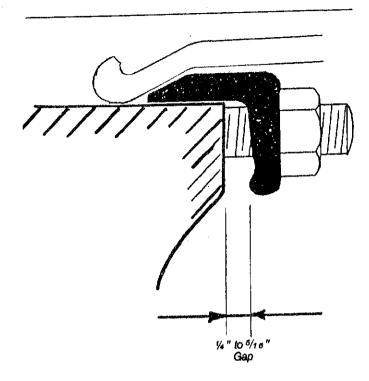
On-front wheels and wide singles, because of the different clamping action, the heel of the clamp must touch the end of the spoke head. The correct fitting of the front clamp assembly is vital to safety. For a better understanding of this we show right and wrong illustrations.
