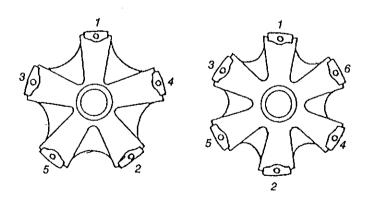
After making sure all mating surfaces, that is the spoke head, rim clamp, spacer and rim, are clean then a good rule of thumb, as to whether the correct spacer and/or clamp is being used is to check the clearance between the end of the spoke and the heel of the clamp at 80% of the recommended torque.
