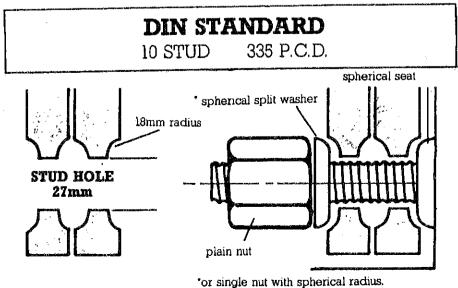
Tightening torque normally recommended for spherical centring wheel fastening by flat collar nut with spherical spring washer is 260 Ft. Lbs (350 Nm) but research in Europe where this standard was first introduced now suggest up to 450 Ft. Lbs - 610 Nm.
