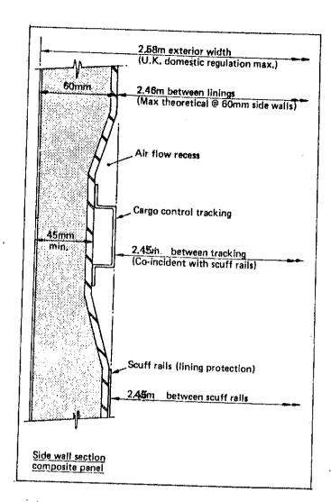
For T.I.P.'s 2.58m wide refrigerated trailers a 60mm side wall with longitudinal recesses to carry cargo-control tracking has been designed. The tracking then does not intrude on the interior width any more than the scuff plates along the bottom of the wall — but the insulation is more effective than if the walls were the minimumallowed 45mm all the way up. The table on the right compares thermal efficiencies (the lower the heat gain figure, the botter).
