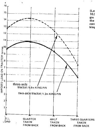
(Left) Why it seems prudent to use the new 10.5-tonne (10.3-ton) drive-axle weight for margin to avoid overloads. As load is removed from the back of the trailer the forward shift of centre of gravity puts extra load through the king pin and on the tractor.
