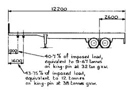
(Above) With dual king pins a tandem-axle trailer can suit either two- or three-axle tractors.
