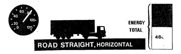
In the same conditions, but at 100 km/h., the proportion due to tyre rolling resistance drops to 38%.
