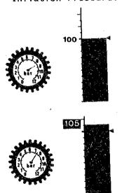
At 80 km/h. on a flat, straight road, and at the nominally correct tyre pressure, our rolling resistance index is 100. If the pressure is reduced by 100 kPa the index increases to 105.
