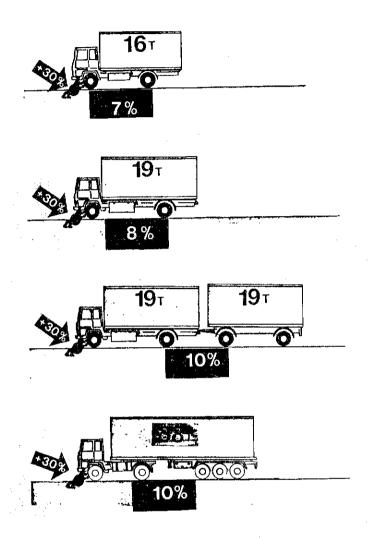
On a straight, flat road surface, at a constant 100 km/h. if the rolling resistance of the tyres, varies by 30%, the fuel consumption can vary by 7 to 10% depending upon the type of vehicle.
