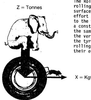
The Rolling Resistance of a tyre rolling on a flat, horizontal surface is characterised by the effort X which must be applied to the wheel axis to maintain a constant speed. It must, at the same time, take into account the vertical load Z supported by the tyre. The value of the rolling resistance is given by their equation:
