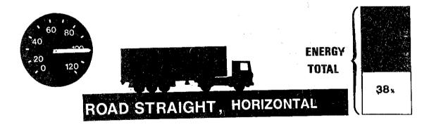
And if the vehicle is on a 1% incline, the proportion drops to 22%.
